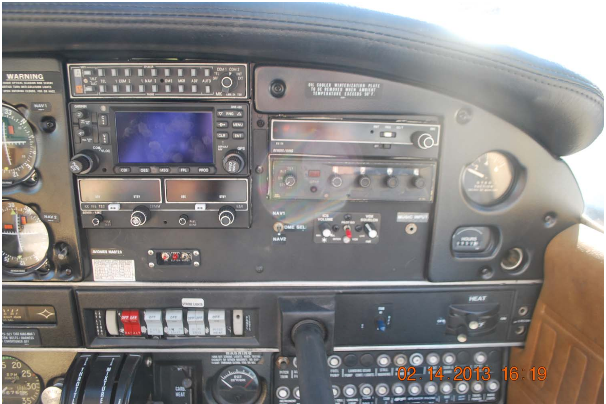
LEFT AVIONICS STACK – Bendix/King KMA24 audio panel and marker beacon receiver; Garmin GNS430 GPS/Comm/Nav; BendixKing KX155 Comm/Nav RIGHT AVIONICS STACK – Bendix/King KN64 DME; Bendix/King KT76A transponder; NAT 4 place intercom. (NOTE: dual glide slope receivers)
