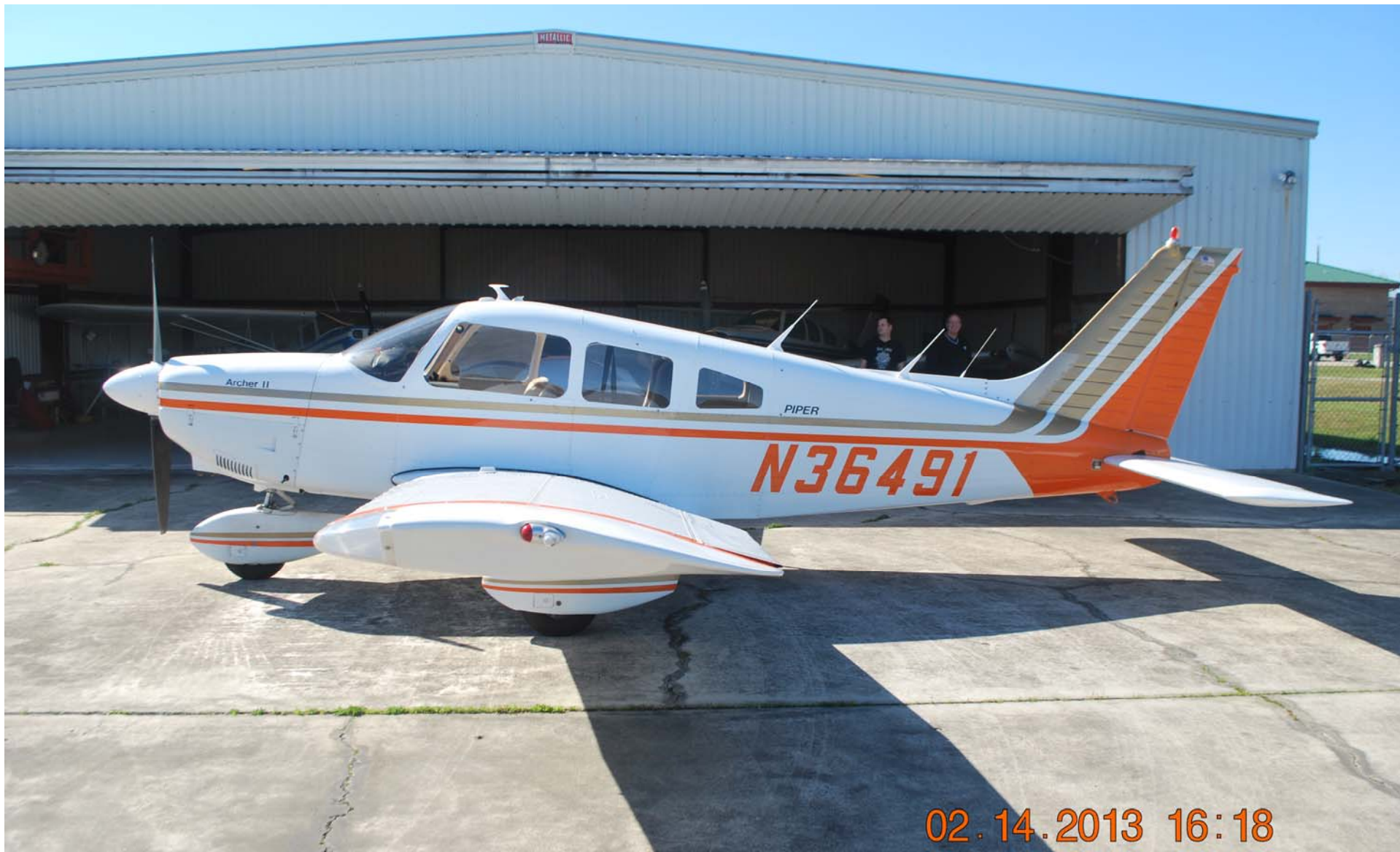
1978 Piper Archer II – airframe total time = 3,700; Lycoming factory overhaul engine with 75 hours since overhaul.
