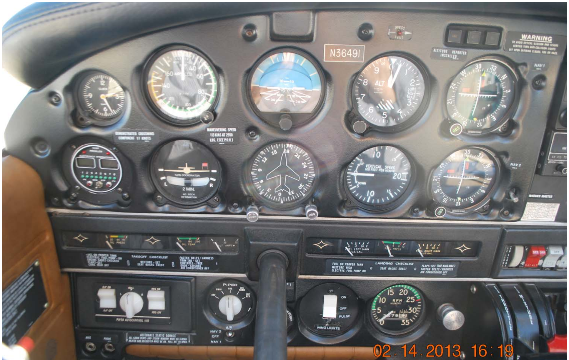
Good old steam gauges. Below clock on left is 4 probe exhaust gas temp and cylinder heat temp system; lower left is AutoFlight single axis autopilot; left of the tach is the controls for the wingtip reco lights – ON/OFF/PULSATING.
