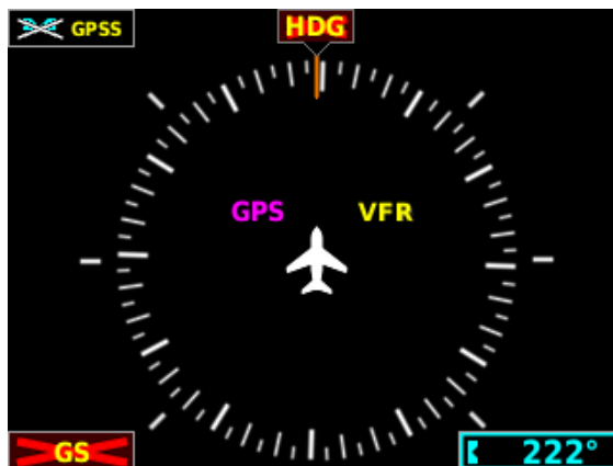
G5 HSI Failure Indications
