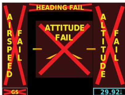
G5 Failure Annunciations
