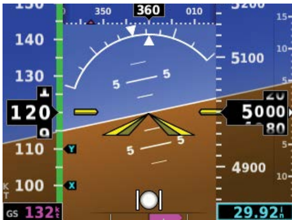
Turn Rate Trend Vector Turn Rate Indicator (Standard Rate Tick Marks) Turn Rate Indicator
