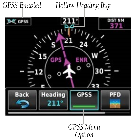
Figure 4-4 GPSS Enabled (HSI Page)
