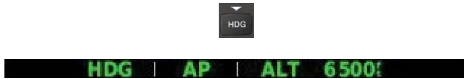
Figure 3-17 Heading Mode Annunciation
