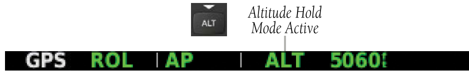
Figure 3-10 Altitude Hold Mode
