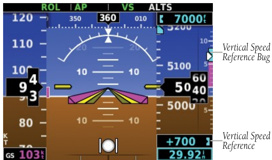
Figure 3-11 Vertical Speed Reference on PFD Page
