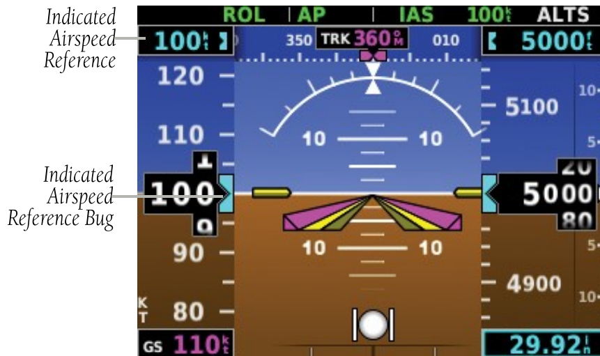
Figure 3-13 Indicated Airspeed Reference on PFD Page
