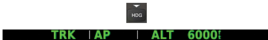
Figure 3-18 Track Mode Annunciation
