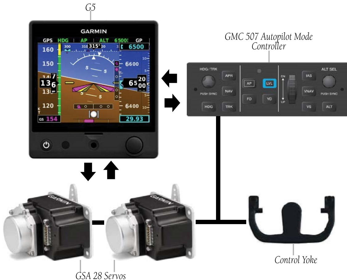
Figure 3-2 Core GFC 500 System
