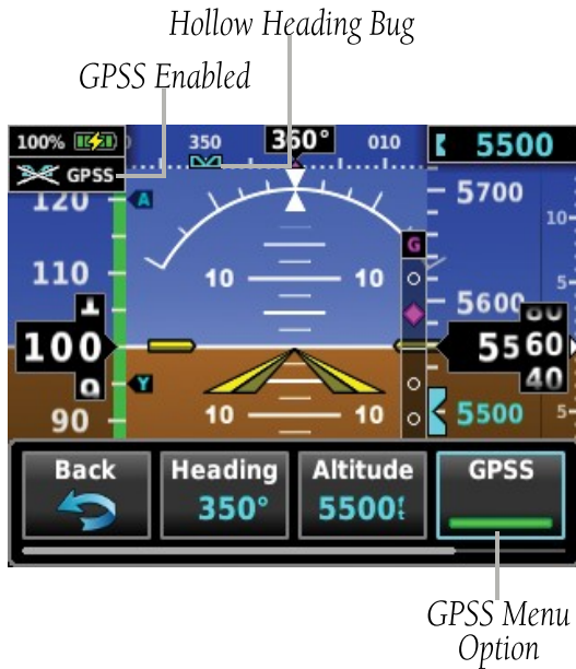
Figure 4-3 GPSS Enabled (PFD Page)
